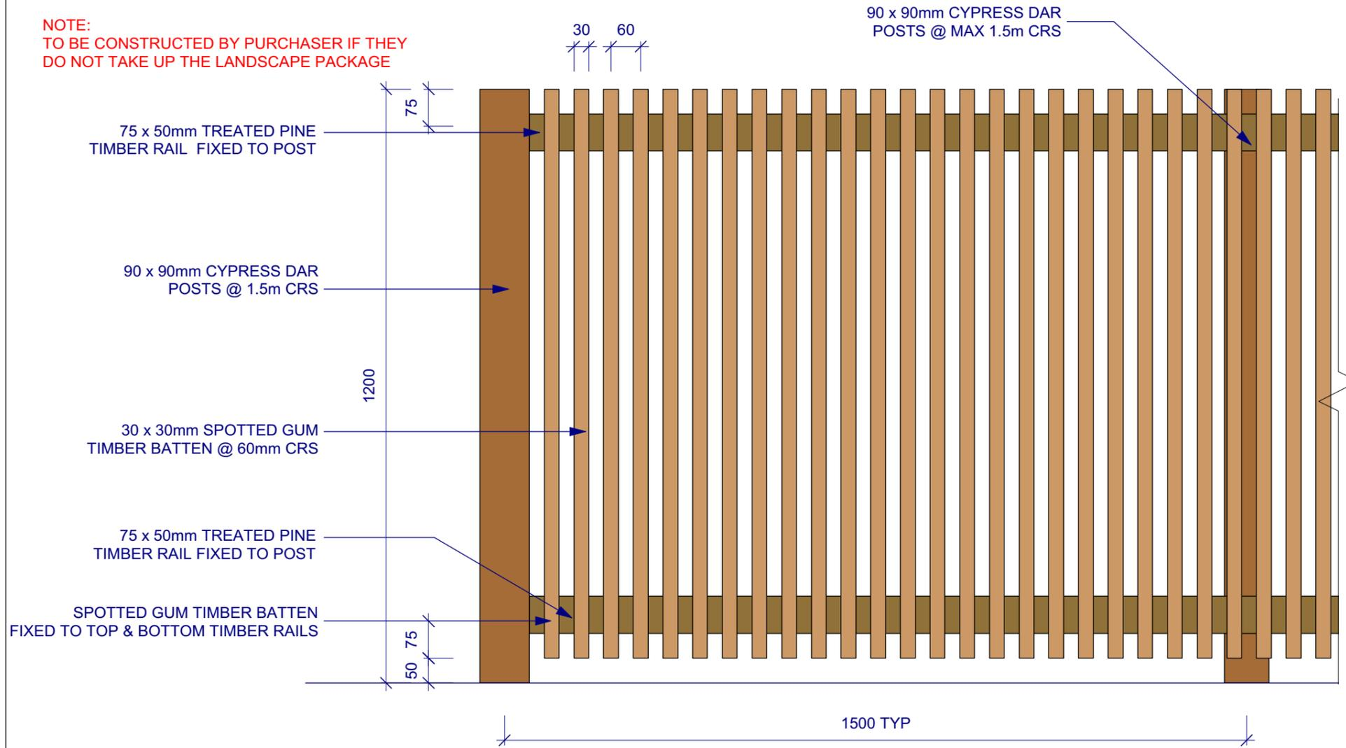
**1** Internal Corral and Driveway Fence - Elevation
